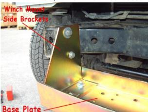
Photograph shows vehicle without winch in place and with bumper removed.
